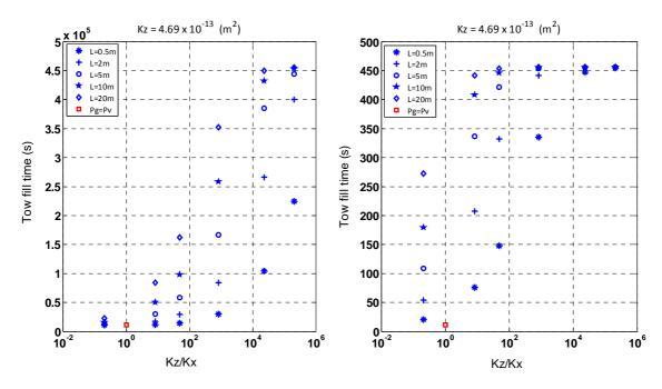
Figure 2: Time to fill a tow of various lengths and permeability ratios at 32°C – left and 130°C - right
